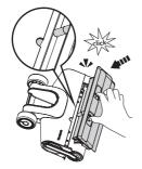
While replacing, always latch the brush cover into place to avoid leakage.
